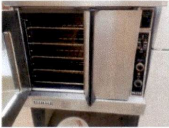
Convection Oven. Excellent for baked goods. Air circulates heat while cooking. On the side panel are the temperature and timer knobs as well as switches for off/on and heat/cooling off settings. Temperature light turn off when the oven is up to temperature. Rack slide in an out for easy removal of hot pans.
