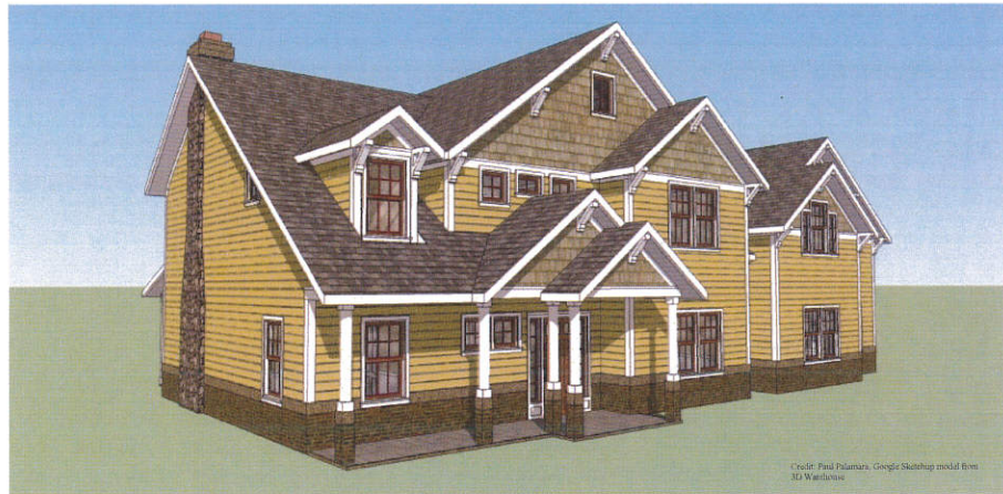
Appropriate wrapping of corners
