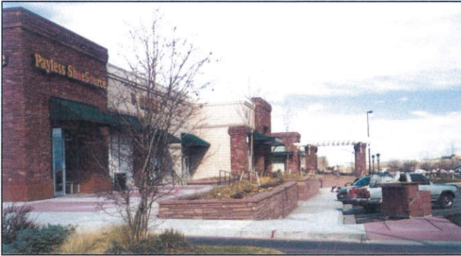
Appropriate use of landscape terraces and retaining walls to address topographic differences between parking areas and stores (left) and along commercial perimeters (right).
