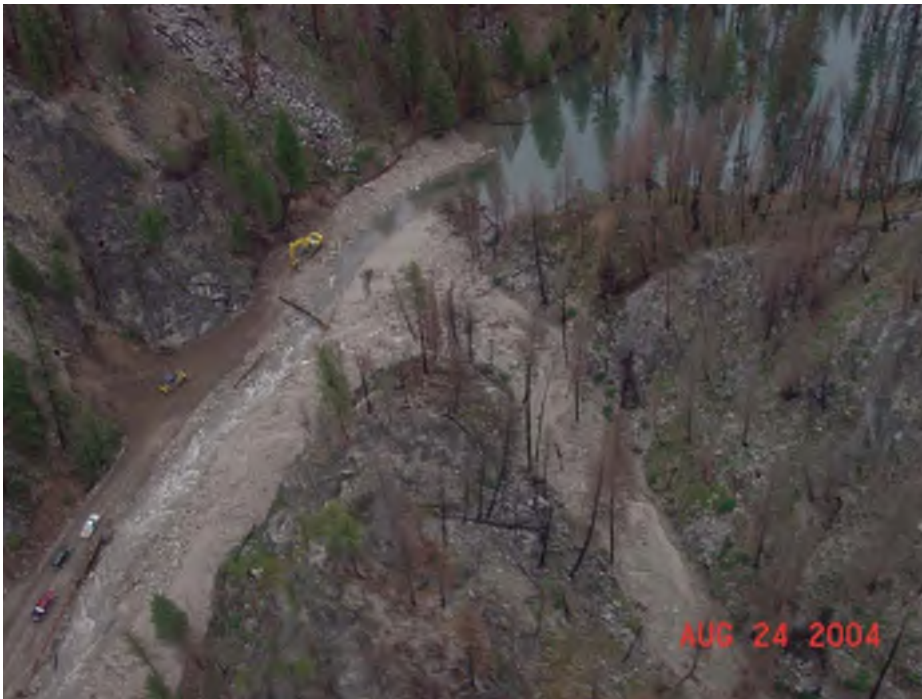
Figure 8. Aerial view of debris-flow deposits in the Middle Fork Boise River. The river was completely dammed at this location, and the road to Atlanta, Idaho, was destroyed. Photograph by Dave Hilgendorf, U.S. Department of Transportation Federal Highway Administration.
